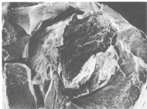
Figure 7 Scanning electron micrograph taken from the fracture surface of the sample shown in Fig. 6 (X 46).
